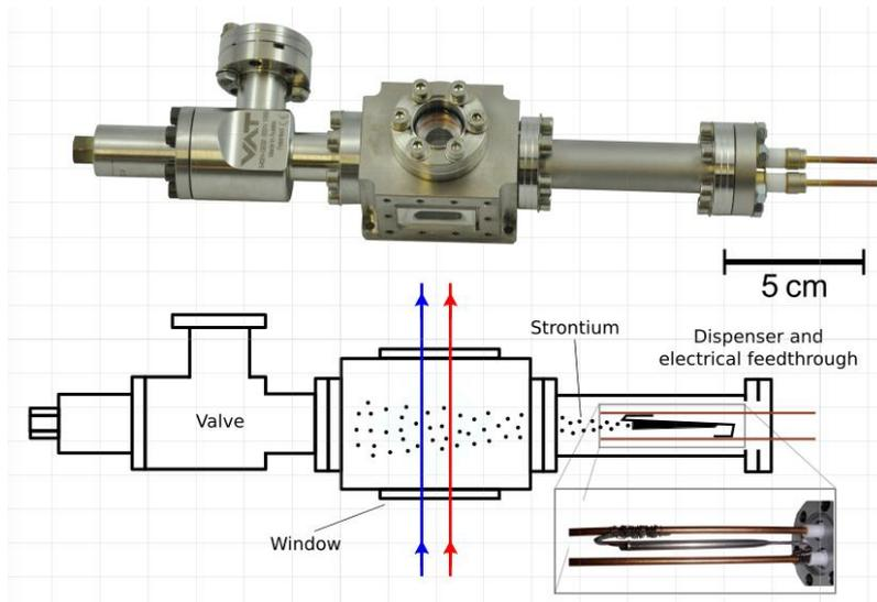
Figure 1: Currently employed spectroscopy cell with a simple strontium source
