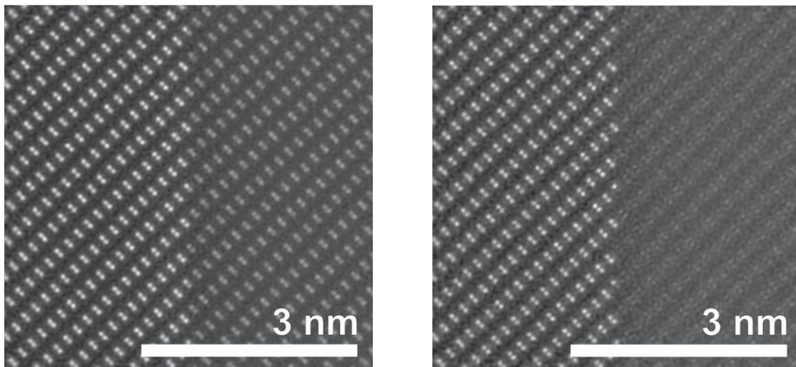
**Fig. 2.** *Left:* Reconstruction of the potential of Si in the middle of the sample. Note how the dumbbells are nicely resolved, despite being absent from the measurements in Fig. 1. *Right:* The reconstructed potential 2.5 nm lower, the right-hand side of the sample doesn't show atoms, thereby indicating there is z-sensitivity.
