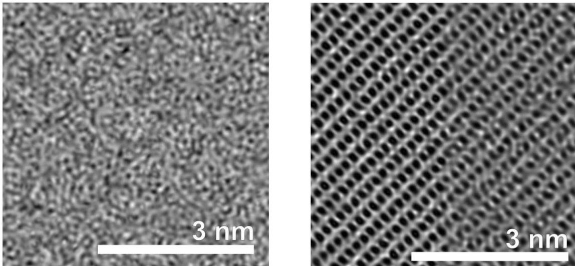
**Fig. 1.** *Left:* Intensity of the illumination with random phases. *Right:* Simulated TEM image of Si dumbbells with random-phase illumination. Note how, compared to Fig. 2, the dumbbells are *not* resolved.
